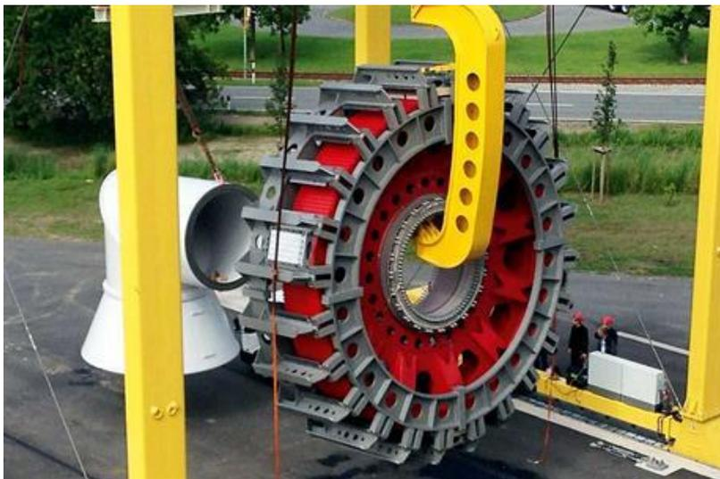
Adjustable - the Venpower generator with 24 separate stator modules and a strong magnetic field could cut Opex costs by 30%
